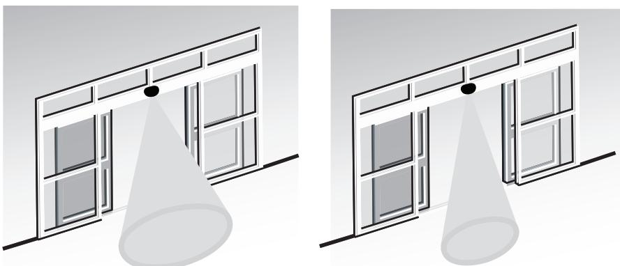
The size of the detection area can be changed using the potentiometer.
